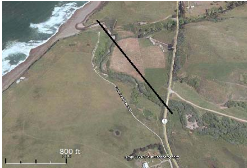
Figure 4. Black line connects known locations of the historically-active San Andreas Fault north and south of Alder Creek Bridge, and trends beneath southern end of Alder Creek Bridge.
