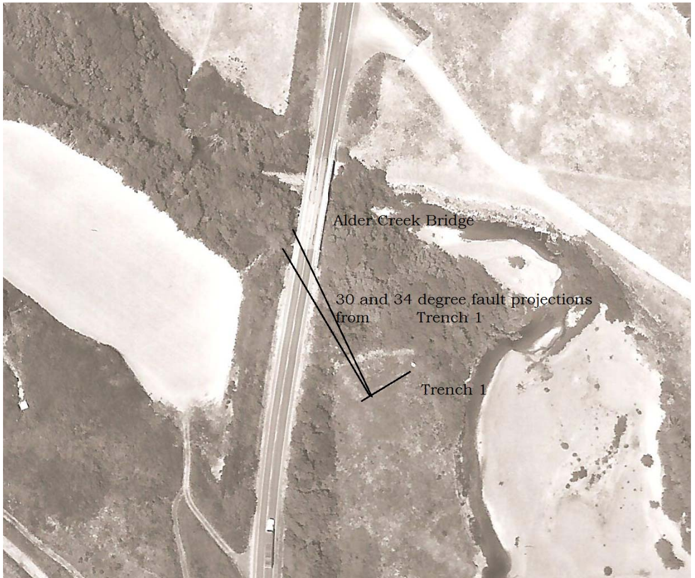
Figure 3. 1999 air photo showing location of 1996 Trench 1 and projection of the San Andreas Fault from Trench 1 towards the bridge. North is at top of image.
